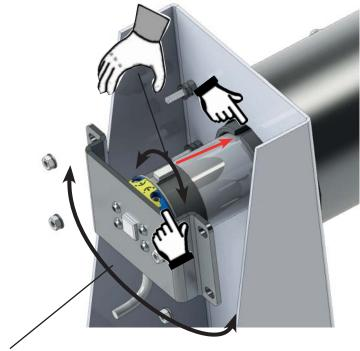
Make small rotating movement with the motor to facilitate the insertion
