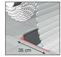
If necessary, cut the sides to ease the passage of the cover and avoid rubbing
