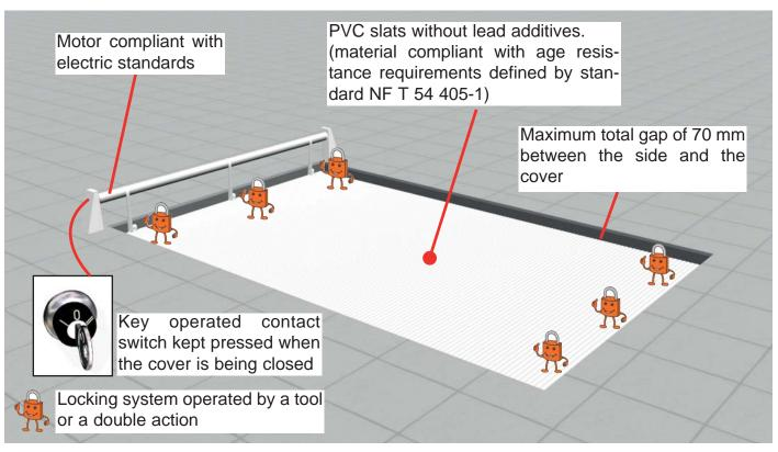
Currently covers with overflows and covers with removable steps on the side are not compliant with standard NF P 90-308.
