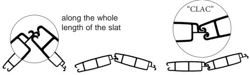
Repeat the movement until all the slats are completely clipped together
